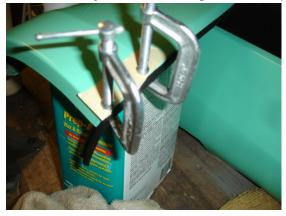
For the rear cladding, start at the back and work forward. You'll have to trim off a small section of beading when you get to the front of the rear cladding. Again, don't stretch it forward. Just push it straight down into the slot. After the weatherstrip adhesive has dried you can clean any excess off using the adhesive remover.
