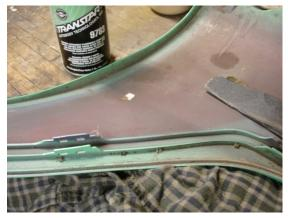
I used a wax and grease remover to clean all the mess off. Then I polished the cladding with various hand polishers and finally the polishing wheel. There were a number of small cuts in the paint. I purchased a pint of enamel paint for touch and went to work. The nice thing about a solid color is that touch up looks great.
