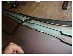
I used some clamps for the front cladding. There is a slot so you'll know it has to be installed in just the right location. The extra beading in the front wraps around so you don't need to trim it.
