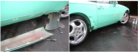
I choose to replace my stone guards. These come off with the application of heat. Then you'll need to get the adhesive off. Once everything is clean I used my polishing wheel and clean the side of the body. Then, pull the stone guards off of their backing and cover the sticky part with a soapywater solution. Then apply to the body and position to the right location. Use a plastic edge to squeeze the soapy water solution out to the sides.
