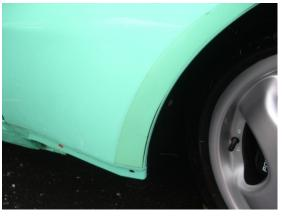
Back to the cladding, after removing the old cladding you'll need to clean out the slots where the new cladding will be installed. Use the adhesive cleaner and some sandpaper to make sure the slots are good and clean.
