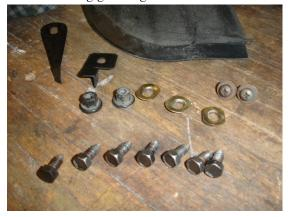
After allowing the beading to dry, turn the cladding pieces over and reinstall the clips. Remember to put the trimmed pin clips in the correct location toward the rear. You're ready to install.
