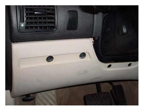
Once the tan colored trim piece above is removed, remove the air vent with the screw as in the right hand side. Remove the "C" clips for the piece of trim. There are TWO on the left hand side. Remove wood trim. First picture below is driver's side trim, second is passenger side.
