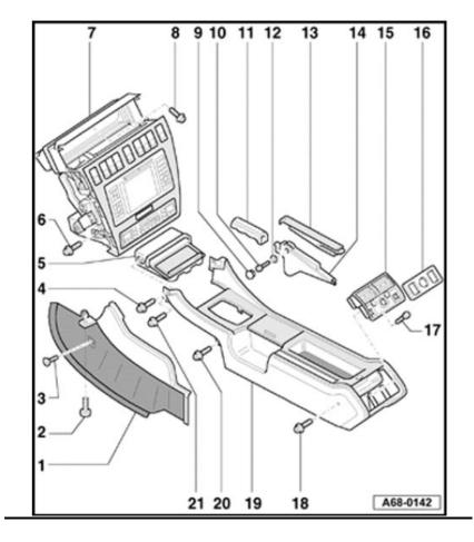
Rear piece by seat heater switches (16): Just gently pry off.
