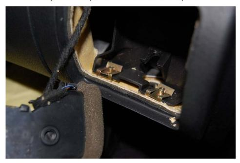
In the picture above, it IS NOT the two screws with the gold backers, it's a screw that sets into the black plastic piece just behind and above it.
