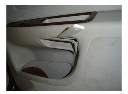
This will expose (2) Phillips head screws (number 12 below), once they are removed, unscrew two Phillips head screws and the wood piece will come out. Disconnect wiring.
