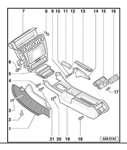
Once the side panels are out of the way, look on each side, behind where the side panels were installed, for the 6mm hex screws and remove them. There are (2) on each side for the wood trim and (2) on each side for the shifter gate aluminum assembly. To make it easy just take them all out.
