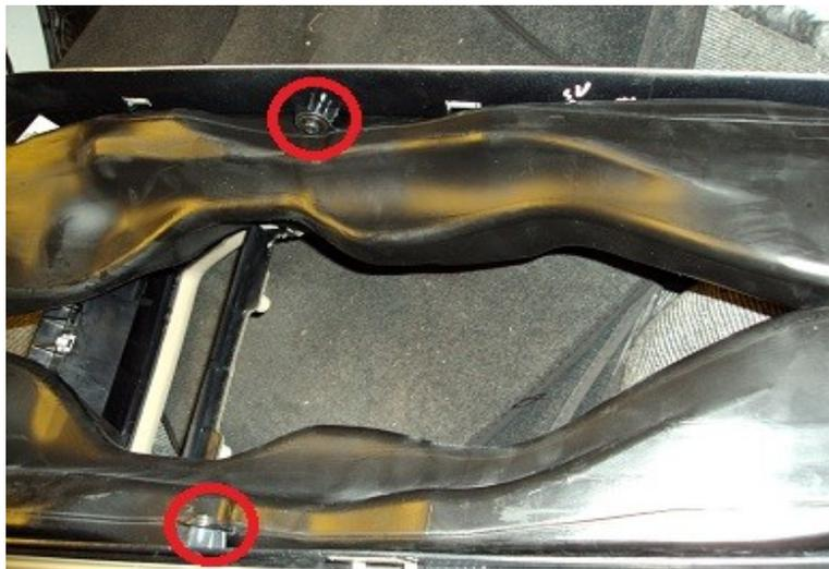
10. Before fitting the new console you need to fit the bracket for the new armrest. Bolts are already there so just remove the cut outs in the foam (see arrow), put the bracket in place and take 4 nuts to attach it. Once in place you can start refitting everything. Nothing strange about this, only make sure the carpet gets in the correct slot
