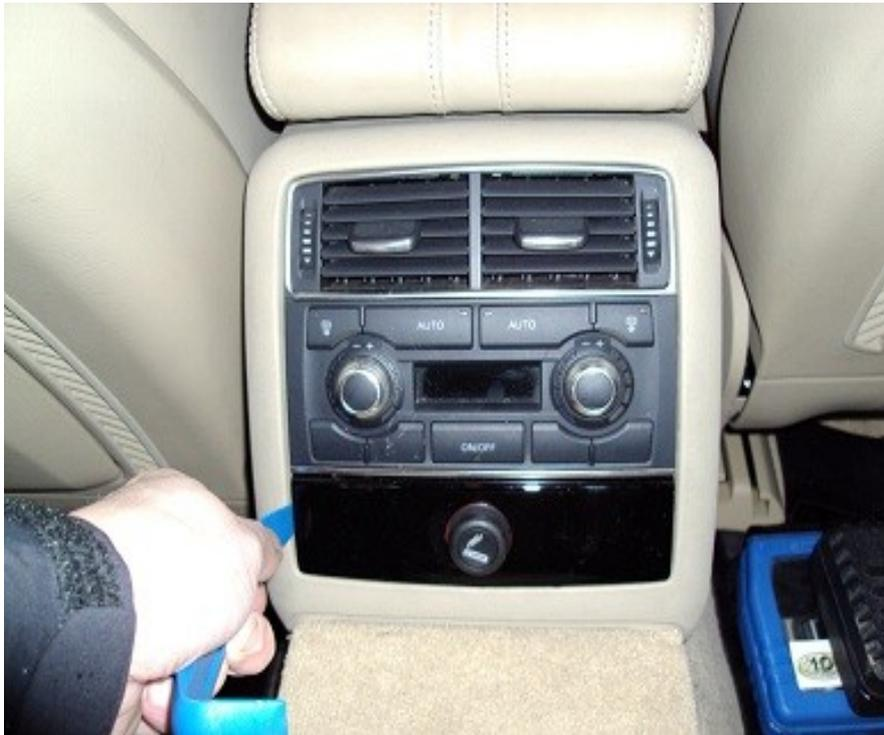
2. Remove the screws (1/side) holding the rear air ducts. Then remove the brackets (3 screws/side) and remove the 2 M8 nuts holding the console to the floor
