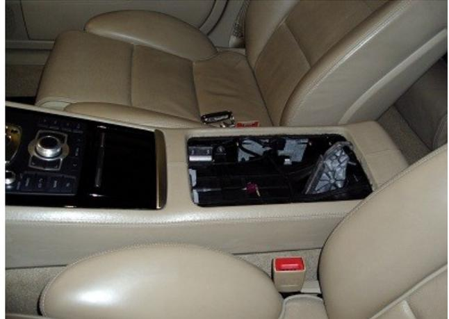
11. Fit the tray, place the rubber seal around bracket and place the armrest in its place. Tighten the 3 T45 screws and finally fit the cover.
