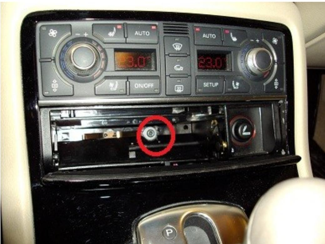
4. Grab the trim in any of the lower corners and carefully lift it up, work your way backwards until it comes loose. Unplug the 3 electrical connectors
