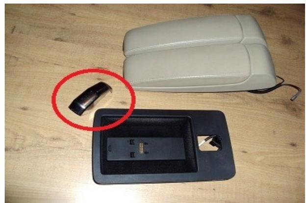
I had no connection for the lights in the armrest storage compartments but just tapped into the rear cigarette light illumination cables. Either use the special gadgets for the purpose or just cut the cables and join all positives with each others and the neg's with each other.
