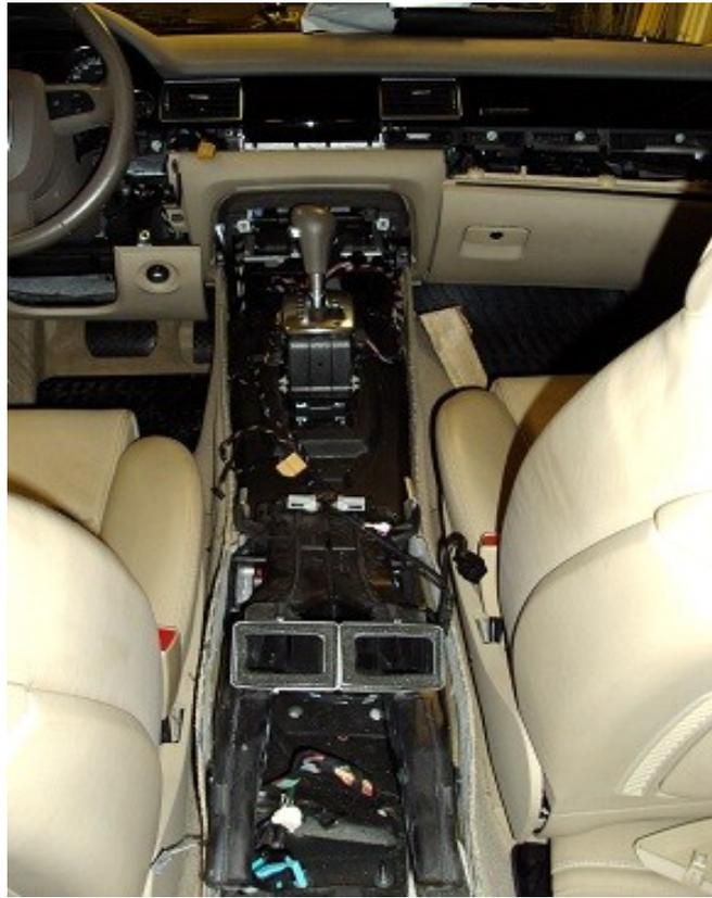
When console's gone, remove the front air ducts and transfer them to the new one.
