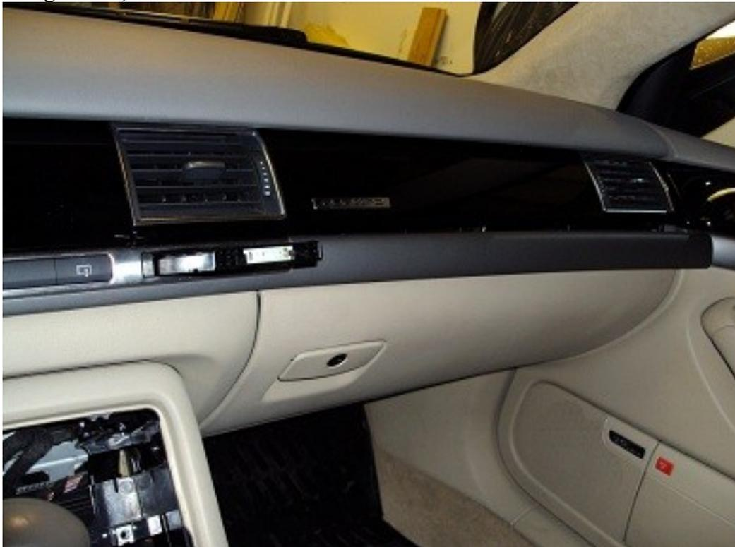
Then take away the fuse box covers on each side of the instrument panel. Remove 2 screws on each side. Now there's only one more screw at the bottom right of the knee panel before you can lower it down enough to get to the last screw holding the console on left side. It's located fairly low down.
