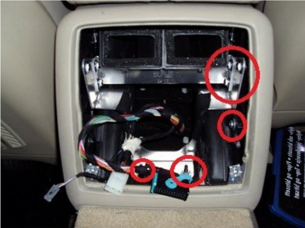
3. Move to the front, pop out the ash tray and remove the T20 screw under it. Remove ash tray compartment.
