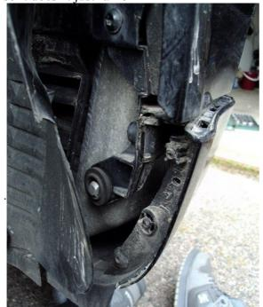
8. Lift off the bumper carefully, there's some wiring and hoses running at the bottom of it and you don't wanna break those. I broke the washer fluid hose....If you remove the 2 large connectors and pop out the wiring/hoses you get some slack to fold the bumper down.
