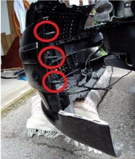
Remove the 2 torx screws and twist the 2 inner quick-lock screws 90 degrees to loosen the fender liner.
