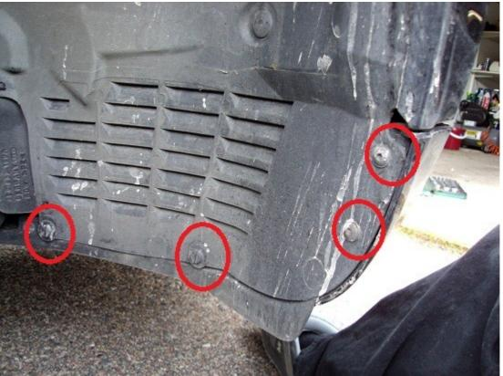
6. Behind the liner it's now possible to see the 3 nuts holding the sides. Remove them using a 10mm socket. It looks like the top one is held with a larger 15mm nut as well but it's not
