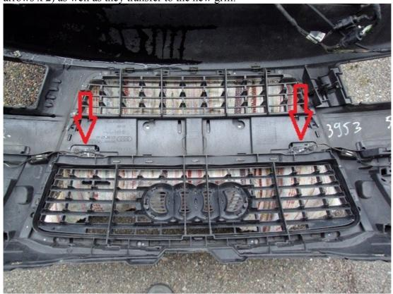
10. Remove the license plate cover. 4 philips screws in the bottom and clipped in on top. If needed, the green notches could be transferred to the new grill. When putting the PDC sensors back, make sure they end up behind the red tab so they are held in place properly.
