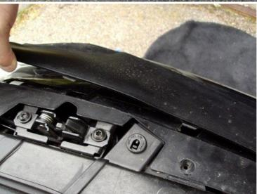
3. Under the trim there are some foam covers on each side of the grill. Use a screwdriver to remove them and remove the T30 screws located under the foam.
