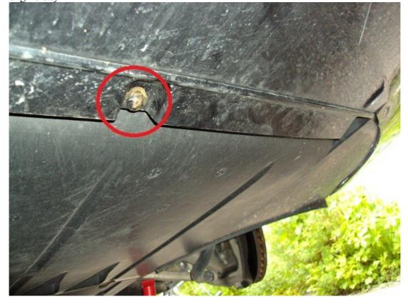
5. Now we got the top and the bottom loose. Time to work on the sides where it sits with 3 studs in the bumper that are held with locking nuts from behind the fender liner. See pic of
