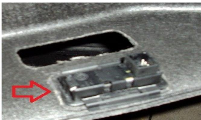
5. Time to remove lid internals. Remove plastic cover over latch and unhook the wire by turning the white plastic disc.
