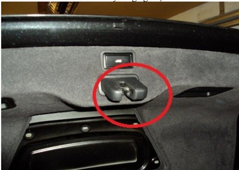
4. Even though you have the non electric lid, the liner is marked for the button so take a sharp knife and cut out for the button frame. Start with a slightly too small one that you trim to a good fit. Starting with a too big hole is not good :-)
