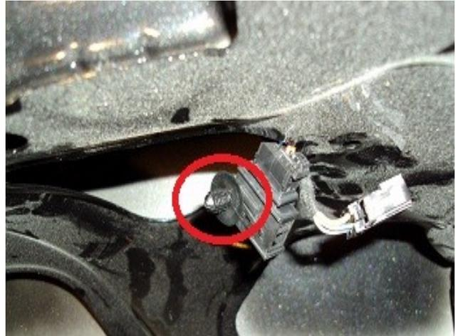
7. If the new lid didn't come with stops you can just drill out the rivets in the old one and transfer the stops and rivet or bolt them to the new lid. Same thing with the white clips for the tool kit. If not in the new lid, just transfer the old ones by pressing them together and then remove.
