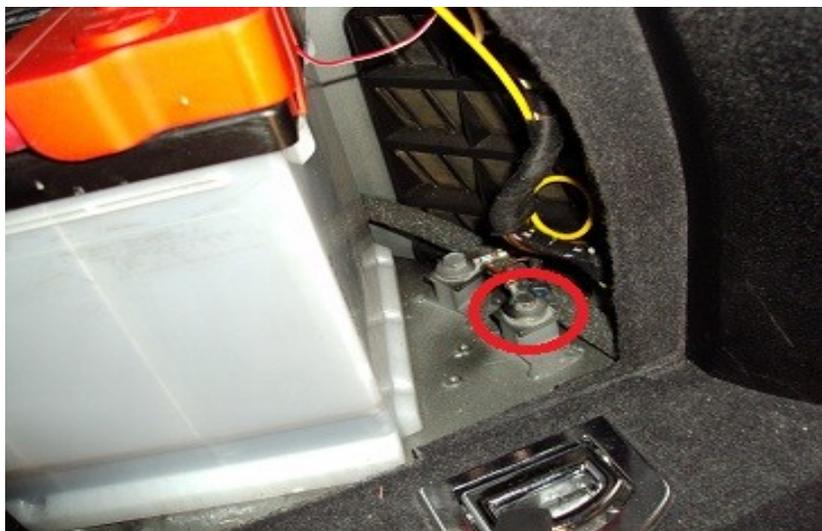
The pin 5 cable is going to positive. I did not want to tap into the main cable harness so I ran it to a free connection on the positive terminal above the battery and put a fuse directly on the cable. I you do the same, just put a ring cable lug on the cable and bolt it to the terminal.
