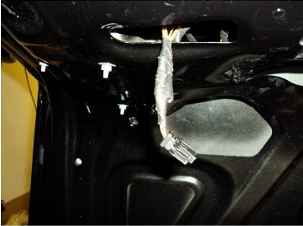
14. Pin 2 on the button is sending the signal to the drive unit so plug a cable there and attach a few ft more, enough to run through the lid, battery compartment and down to the drive unit. Use some grease, 5-56 or similar to make it easier to slide through bushing etc. The part running through the hinge was too tight so I just hockey taped it outside the other cables
