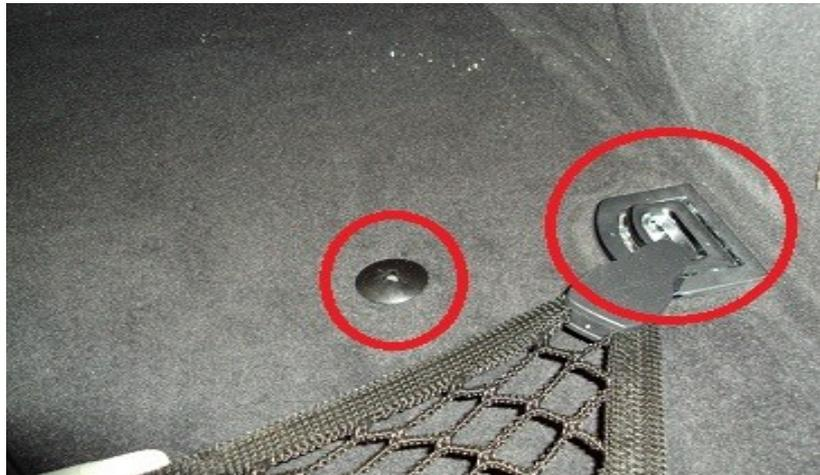
The plastic trunk sill needs to go so take a fine screwdriver to get one plastic plug out. Once gone you can remove the other one as well, see below pic. Repeat on the other 2 plugs. Once plugs are gone, the sill sits with some clips so pull carefully upwards to remove it
