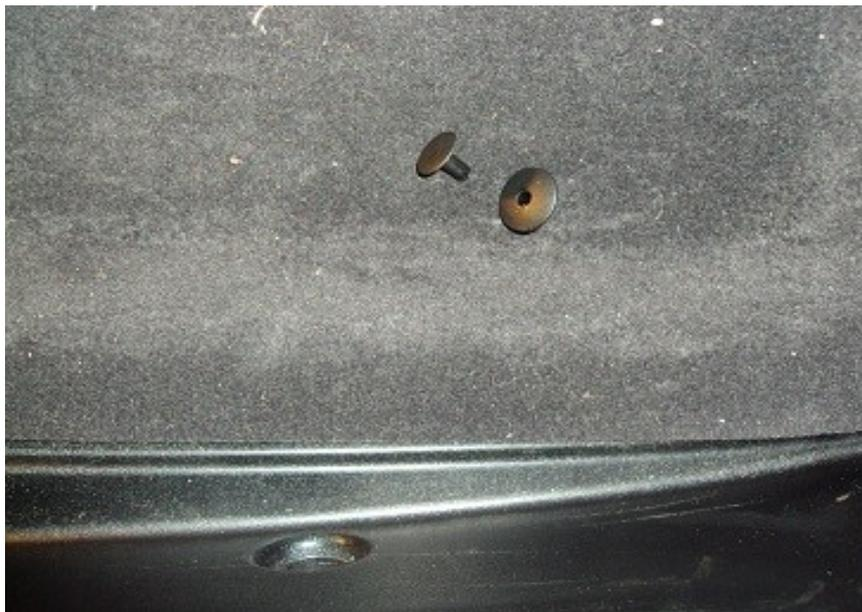
When the sill is gone you can remove the right side trunk liner. It sits with 2 plastic clips around the battery compartment.
