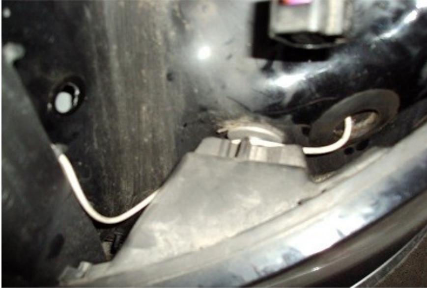
16. Take the drive unit connector and plug 2,5mm cables to pin 1, 2, 5 och 6. The cable from the trunk lid should now be connected to the pin 2 cable on the drive unit. Then crimp a ring cable lug to the drive unit pin 6 cable and bolt it to one of the earthing point next to the battery.
