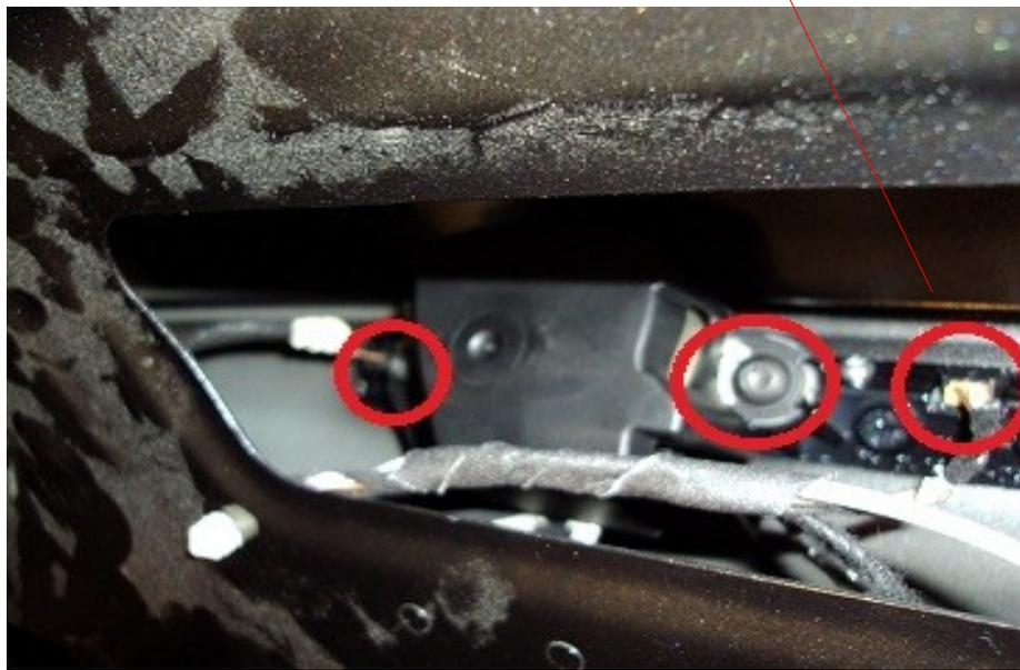
If the new lid doesn't come with the exterior handle just transfer the old one by removing 4 torx screws to get it loose.
