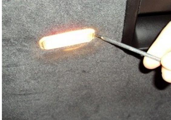
3. Grab the plastic cover over latch and pull it off. Now the trunk liner only sits with clips so pull carefully around the liner and it will pop out so you can remove the whole thing. (Picture taken after I assembled everything again)
