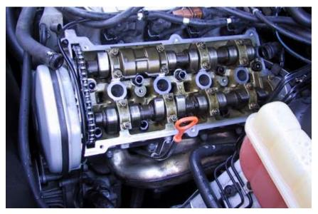
Left hand valve train. Note valve cover breather hose removed on top of timing belt cover. When removing this hose, gently push the hose off the fitting and reuse the clamps by leaving them in place.
