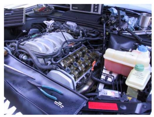
After examining the old leaking gaskets with an eye loupe, it appears that they were leaking on the valve cover side, perhaps due to the unmachined (rough) edge. This is why the "brush in a can" is suggested as a sealer on this surface. The automotive silicone sealer used at the 90 degree cam carrier to cylinder head junction was also used at the factory during initial assembly. The "brush in a can" is an addition to the original factory set up.
