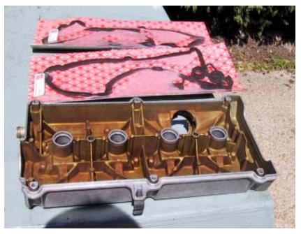
Backside of Audi A8 valve cover and replacement gaskets. When replacing the gasket, ensure the valve cover and cylinder head are completely cleaned before installation of new gaskets.
