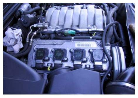
Right hand valve cover. Note each coil is bolted in place, fuel lines are above and on the left, engine throttle body is stuffed with rag, and valve cover breather hose is on the front end of the valve cover.
