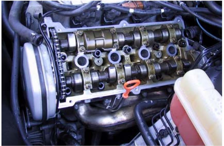
*Left hand valve train. Note valve cover breather hose removed on top of timing belt cover. When removing this hose, gently push the hose off the fitting and reuse the clamps by leaving them in place.*
