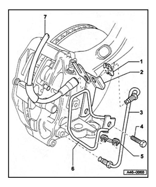
As of implementation of the combination sport suspension - 8J x 18 wheel, the brake caliper housing of the front brake is equipped with an additional bracket (for all vehicles). If the 8J x 18 wheel is retrofitted and there is no bracket at the brake caliper housing, retrofit according to illustration.
